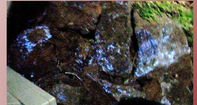
UV lamping at night reveals high grade scheelite (tungsten mineral) in trenches
